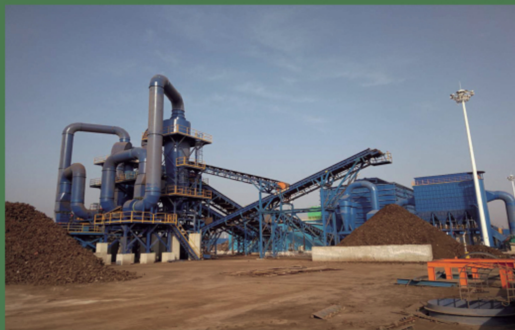
河南安阳11000匹马力项目，全球最高马力废钢破碎机，创造破碎机产能新记录，每小时产能轻松突破400吨。 The shredder project with 11,000HP in Anyang, Henan, is the highest horsepower scrap shredder in the world, setting a new record for shredding capacity, which can easily exceed 400 tons per hour.
