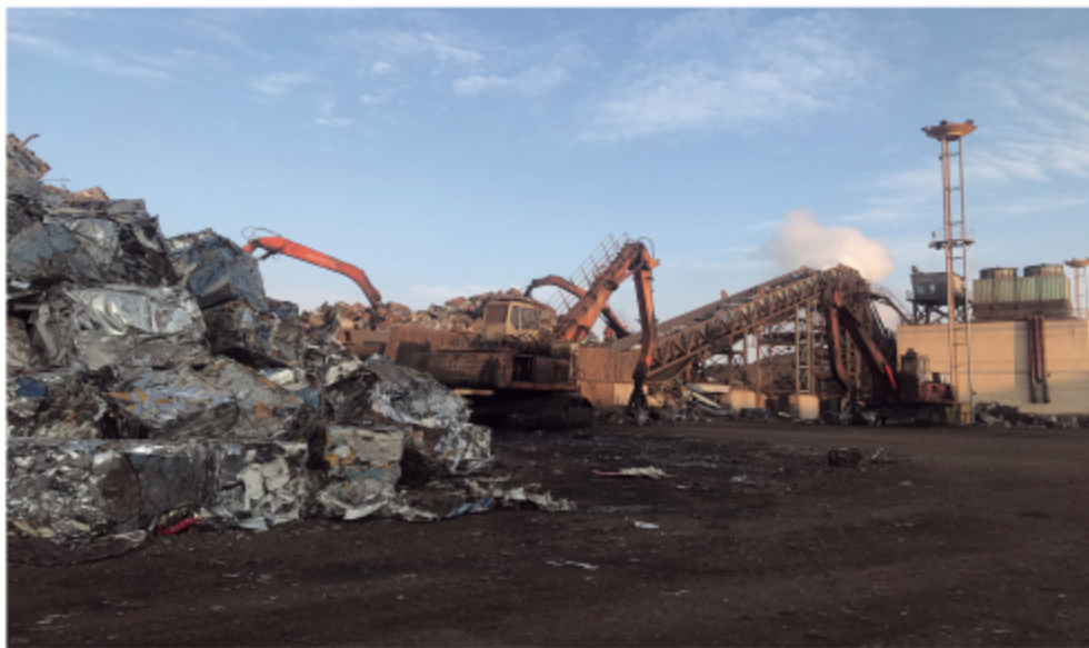
江苏张家港破碎生产线直接破碎废钢压块，被客户誉为“真正的钢铁侠” The shredding production plants in Jiangsu Sha-steel can shred the bales directly, known as the "real iron man" by the customer.
