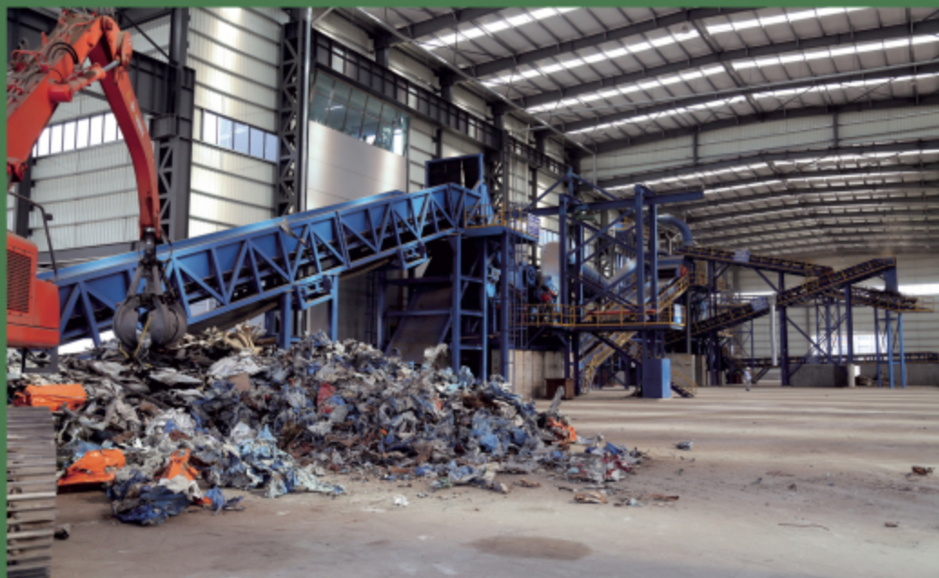
2018年投产运行的纽维尔3000匹马力破碎线，可直接破碎报废整车，年产能高达20万吨。 The Newell shredder production line with 3000HP, which was put into operation in 2018, can shred the scrapped automobiles directly, and the annual capacity can reach 200,000 tons.
