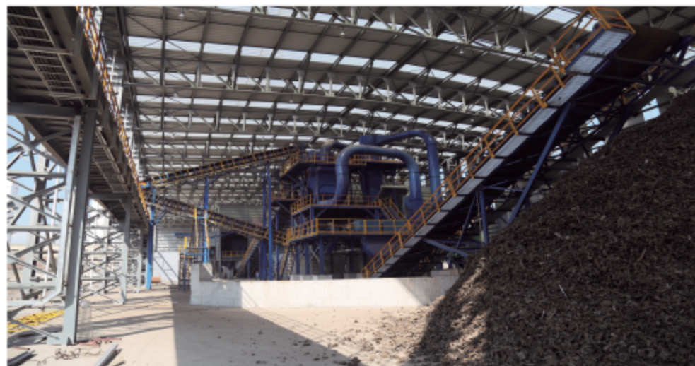
100 SXS型 6000匹马力废钢破碎生产线实景 Reality images of 100 SXS scrap shredding production line with 6000HP
